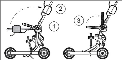
2. Squeeze the cutting depth adjustment handle (3) and move into upright working position.
